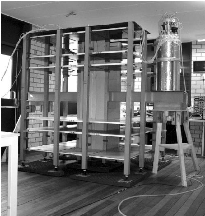
Figure 5.2. Characterization coil set and cryostat containing the gradiometer. During gradiometer balancing the cryostat is slid into the central pillar of the characterization coil set.
